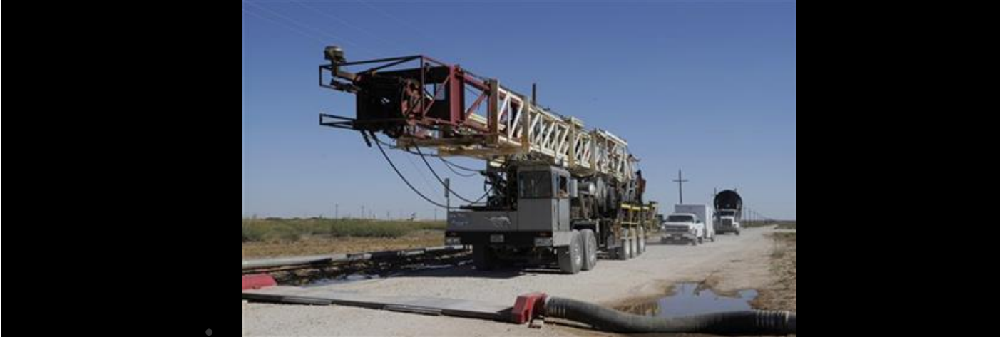
A drilling rig used for hydraulic fracturing is trucked across a water hose at a drill site Sept. 24, 2013, in Midland, Texas. The drilling method known as fracking uses huge amounts of high-pressure, chemical-laced water to free oil and natural gas trapped deep in underground rocks. With fresh water not as plentiful companies have been looking for ways to recycle their waste. (AP Photo/Pat Sullivan)
